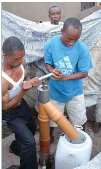
Figure 1. The 'Gulper' being used to empty a pit latrine hygienically in a shantytown in Dar es Salaam, Tanzania. Being small, light and portable, it can be used in confined spaces and on premises only reachable down narrow, winding alleys which do not allow access by vehicles. It is also affordable to local artisans.
