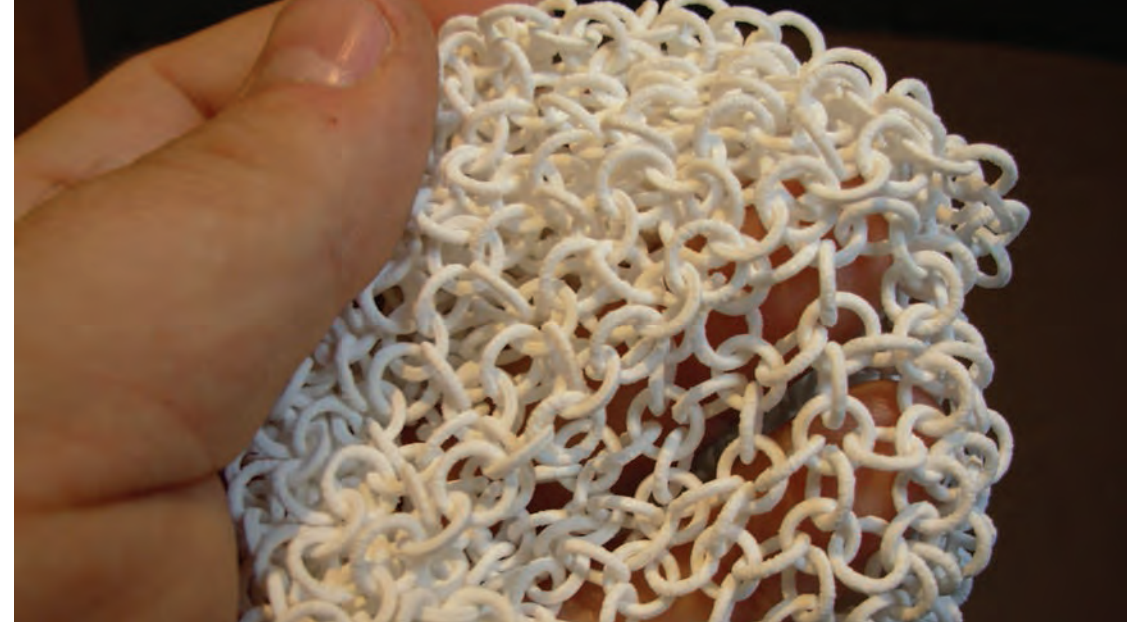
Photo: Selective laser sintered (SLS) chainlink © Econolyst
