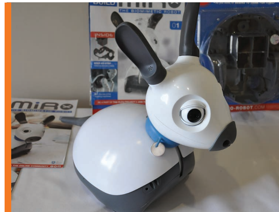
MIRO is a biomimetic robot created by the University of Sheffield that copies the behaviour of animals. It can learn from its interactions and can become loyal to its owner and respond to their voice
