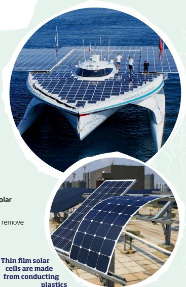
The sails of the yacht provide for a significantly larger area; however, silicon solar panels cannot be used because the silicon will break when bent.
