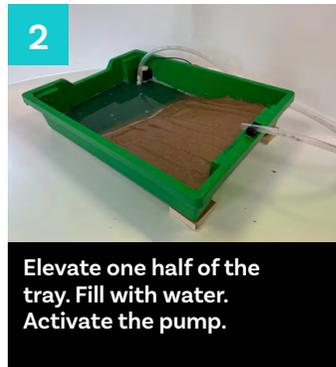
Elevate one half of the tray. Fill with water. Activate the pump.
