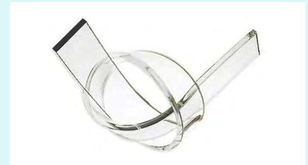
**Cold-forming plastic is a smart material** that can be shaped by hand at room temperature. It is a **shape-memory** polymer, so it will return to its original shape when heated - e.g. in hot water or with a hair dryer.
