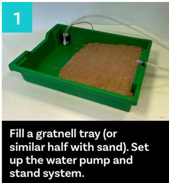
Fill a grate tray (or similar half with sand). Set up the water pump and stand system.
