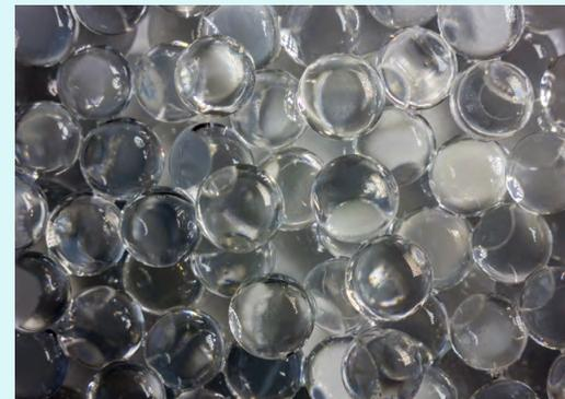
**Hydrogels** are materials that can swell in water, holding a large amount whilst still maintaining its structure.
