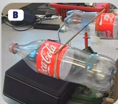
Balance the centre of the dowel rod on the pivot point. Now play the recorded bottle sound through a speaker towards the bottles and see what happens
