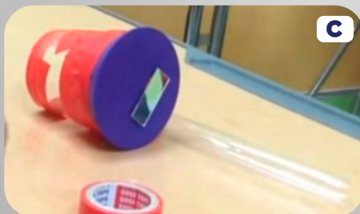
Stick the mirrored piece to the centre of the balloon drum
