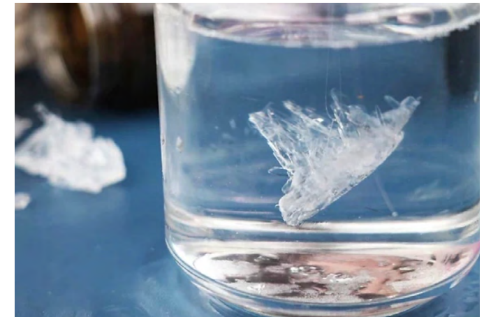
Suspend the seed crystal in your supersaturated solution.
