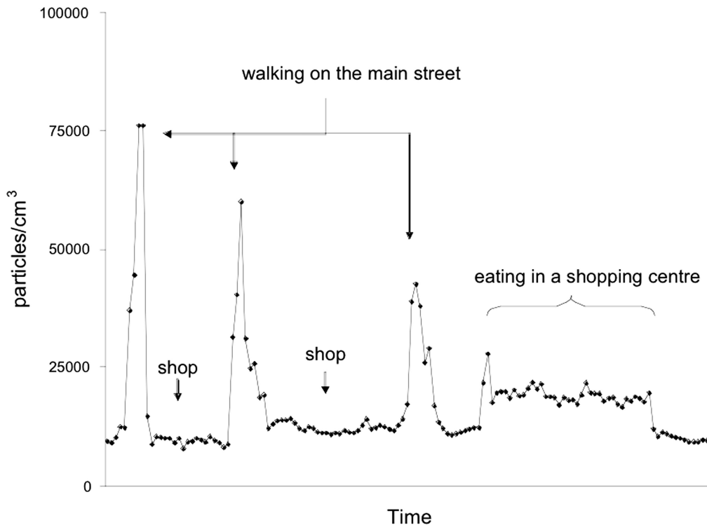
Figure 5.4 Exposure to particles over the course of a four hours spent in Aberdeen City centre. Measurements were taken using a PTrak continuous particle counter which counts all particles below 500nm, though in ambient air the very large majority are below 100nm. (Data collected by Martine Dennekamp, University of Aberdeen)
