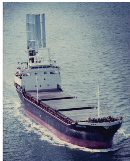
Figure 3.14 mv Ashington wing sail application © Mercator Media 2013
