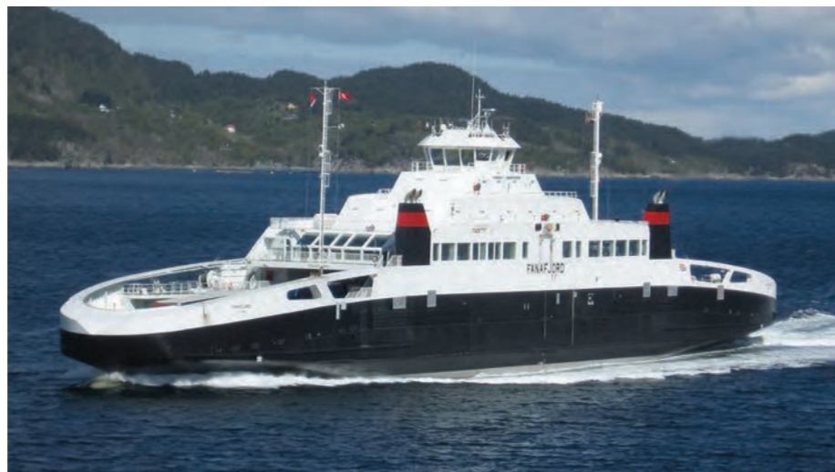
Figure 3.4 MF Fanaffjord : an LNG fuelled ferry [Courtesy A. Greig]
