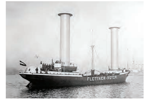
Figure 3.12 The Flettner rotor ship Baden-Baden , formerly the Buckau . Image courtesy of Wikimedia Commons
