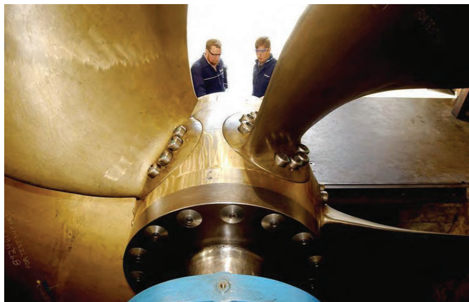
Figure 4.2 Controllable pitch propeller testing. This photograph is reproduced with the permission of Rolls-Royce plc, © Rolls-Royce plc 2013
