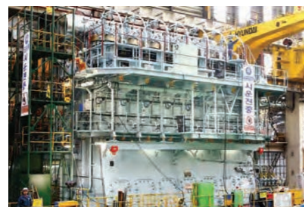
a. Low speed marine diesel engine, the Wärtsilä RT-flex82T version B main engine © Wärtsilä
