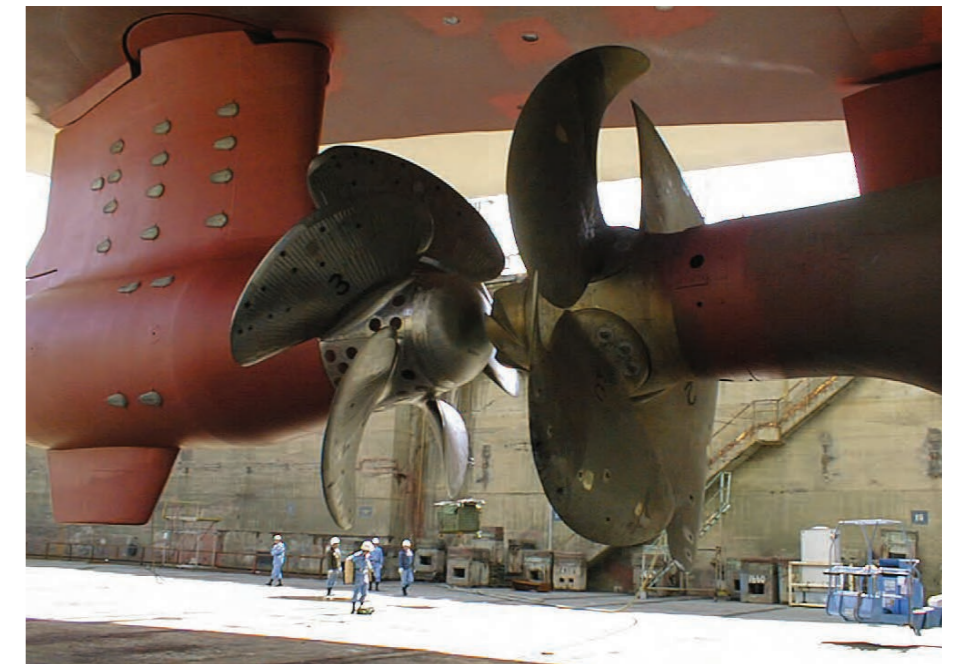
Figure 4.3 A contra-rotating propeller system incorporating a podded propulsor [Courtesy ABB]
